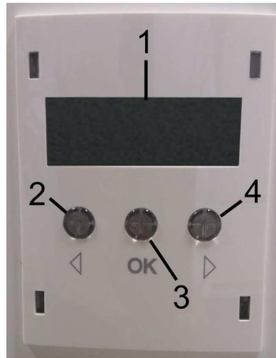
Fig. 2.1 Display and Control panel
